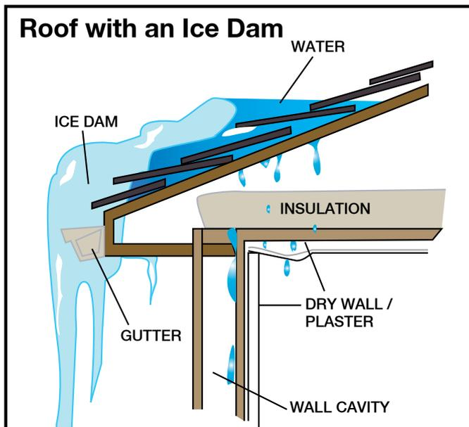
**For many older and larger buildings active management of the temperature profile within the loft or attic space immediately below the roof is important to prevent water ingress through the formation of ice dams. This problem is less prevalent in modern factories or commercial buildings where building construction standards are more resistant to water ingress and the drainage channels from roofs are more free flowing and less prone to ice blockage.**
