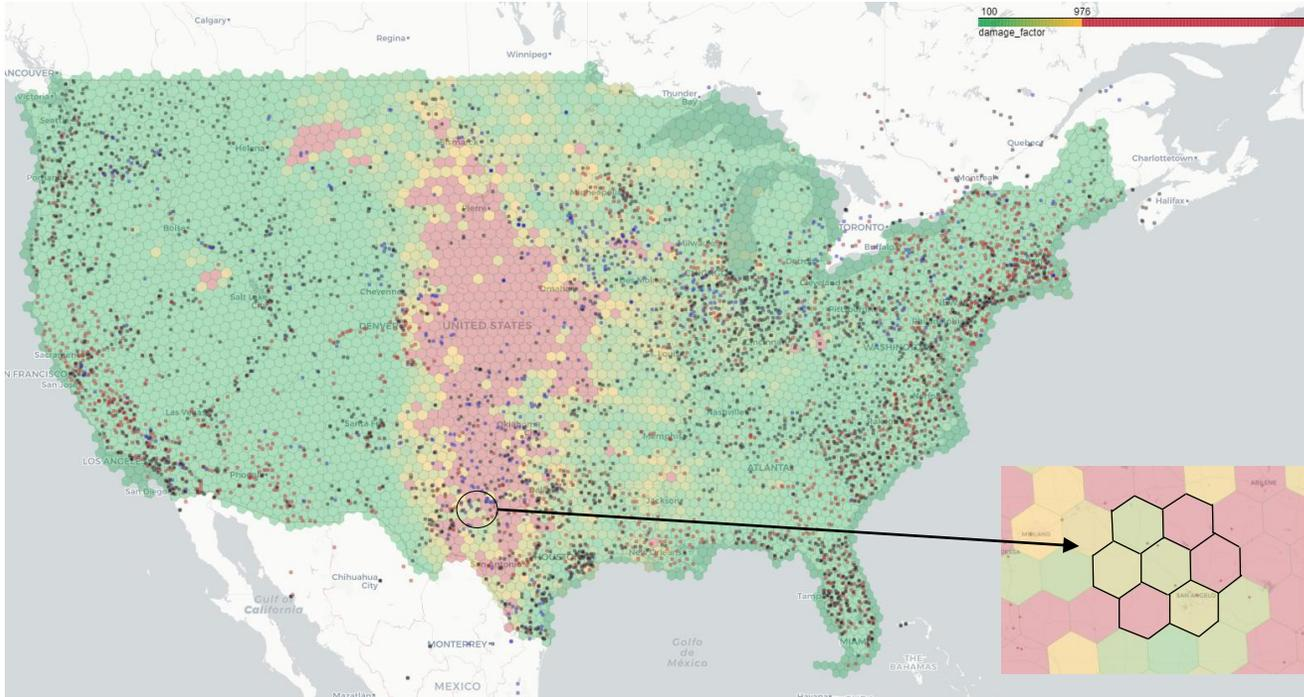
Blue dots – Wind farms, Red dots – Solar farms. Black dots – all other occupancy types. Plotted Exposure for Sustainable energies. Colour is based on damage factor. Which uses the size of the hail sized scaled up by a factor based on what damage it could do to assets, particular solar.
