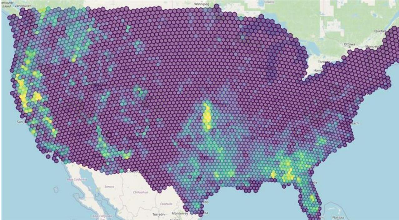
Hexagon geospatial map can be used as a primary aggregation tool with overlays being drawn from tools such as NOAA datasets.
